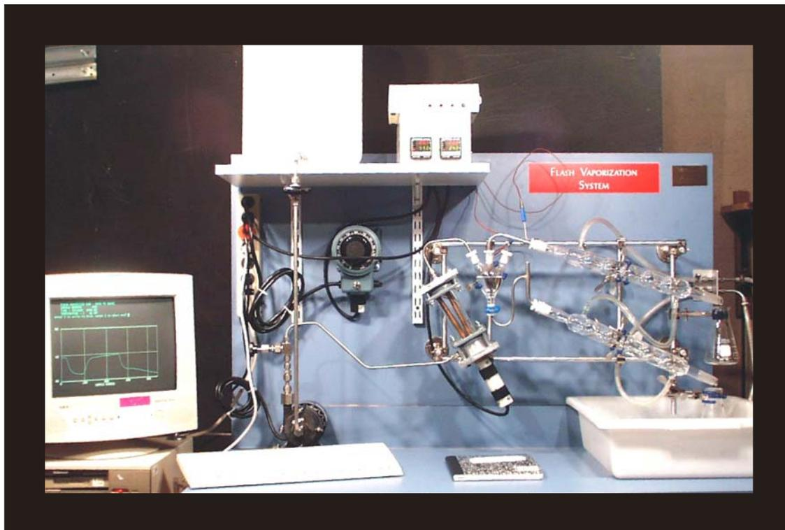
*Flash vaporization experiment, showing 20 liter feed tank with ball valve, magnetic drive centrifugal pump, flow control needle valve, glass vaporizer with internal 1000 W heater, glass flash vessel with overflow line, bottoms cooler, overheads condenser, bottoms and overheads sample flasks. Note also two temperature indicator/controllers and A1000 converter box, liquid and vapor thermocouples, liquid and vapor thermocouples, variable transformer for setting power level.*
