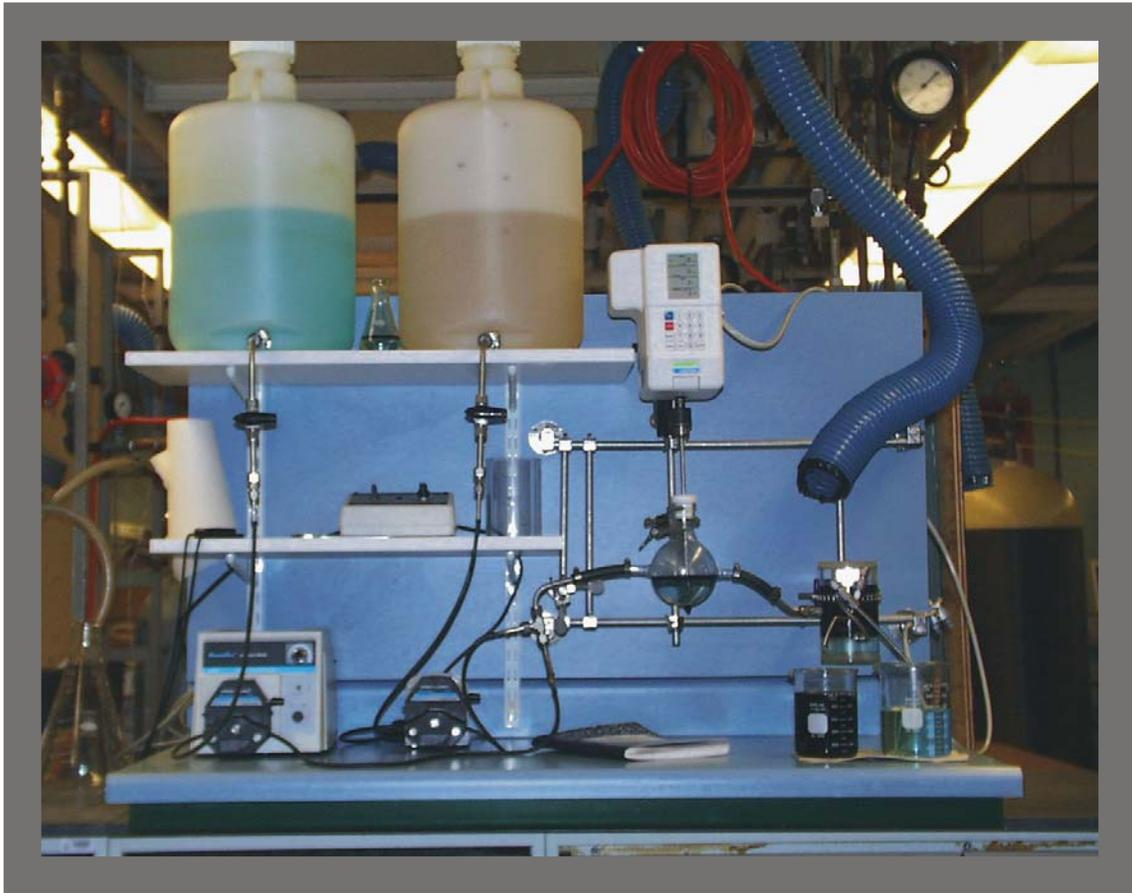
*Photograph of the copper liquid-liquid extraction experiment, showing the copper and LIX + kerosine feed tanks, roller pumps with speed controllers, mixer-settler, variable speed stirrer, and raffinate and extract sample collection. The aqueous raffinate phase is analyzed for copper by a spectrophotometer.*
