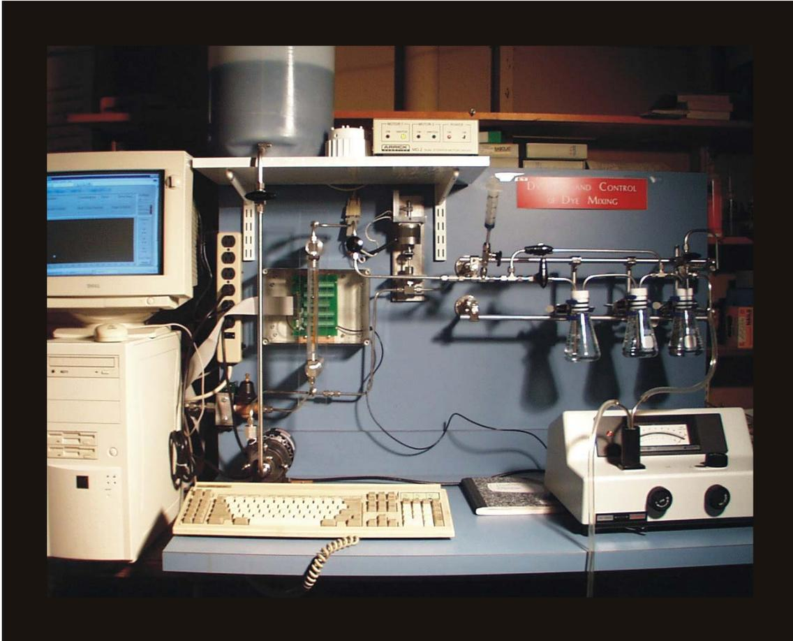
*Dye mixer dynamics and control experiment, showing water pressure regulator, rotameter, dye solution feed tank, magnetic drive centrifugal pump, power strip with GFCI protector, terminal board for NI A/D board, stepper-motor driven needle valve, three flask flow system with ball valves, dye injection syringe, spectrophotometer with flow cuvette and connection to terminal board, stepper-motor control box, computer with National Instruments A/D board and LabVIEW software.*
